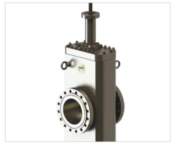
MV7-F-SS Subsea Forged Gate Valve 10" CL.300 RTJ Forged Body LTCS with SS weld overlay on all wetted parts, Duplex trim, TCC hardfacing, lipseals High pressure gas testing, 35m depth, Malaysia
